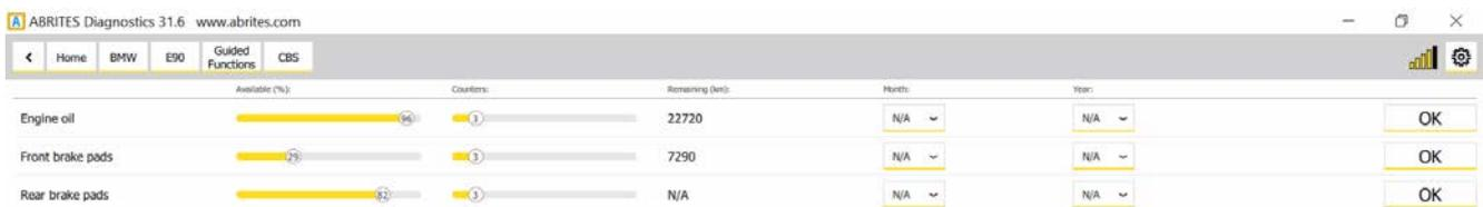
The screenshot shows the 'Guided Functions' section of the Abrites Diagnostics software. It displays a table of service intervals with columns for 'Available (%)', 'Counters', 'Remaining (km)', 'Month', and 'Year'. Each row includes an 'OK' button.
