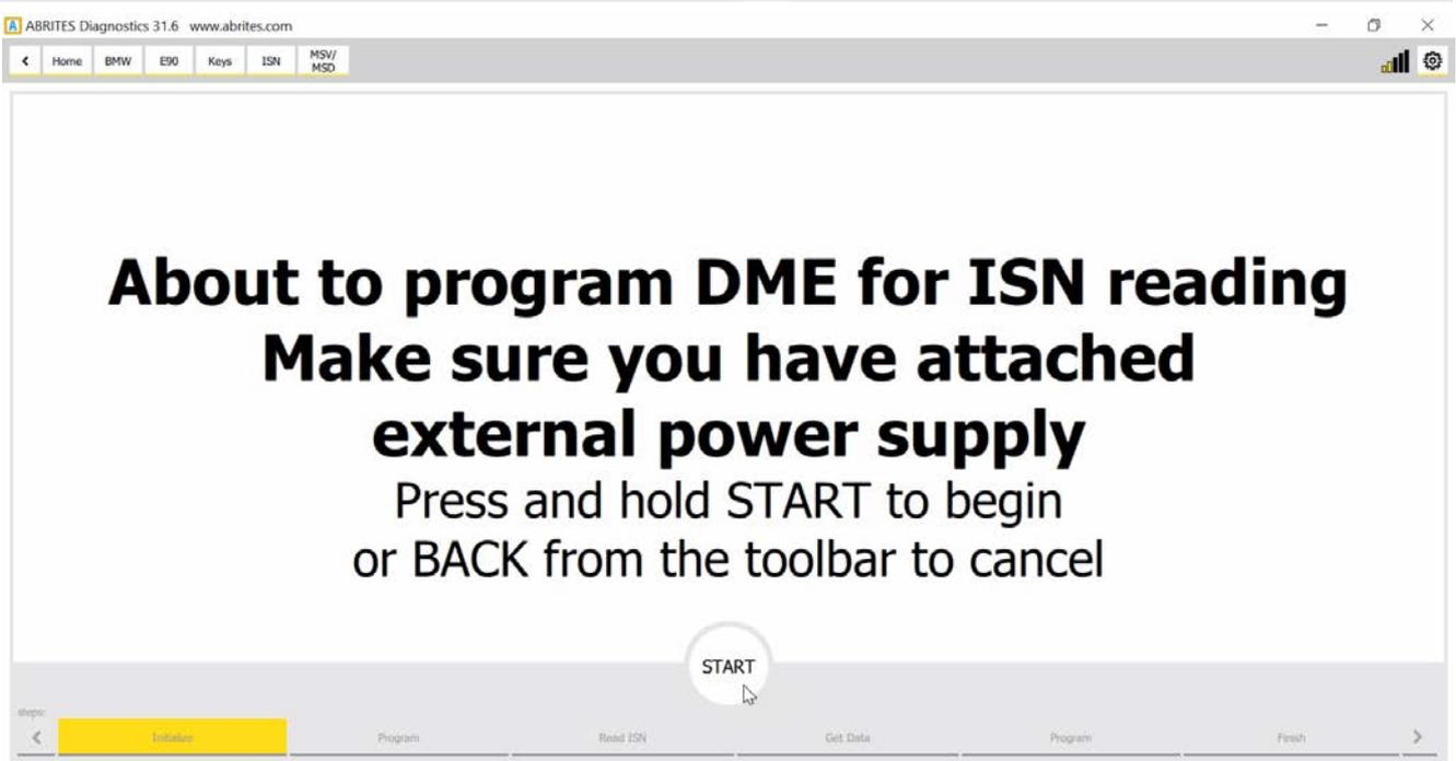
The Start button needs to be pressed and held down as an additional safety precaution. The other buttons in the keys menu will allow for the synchronization of the CAS, DME and other modules where it is needed during and after key learning.
